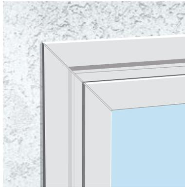
This configuration comes with a flange on the exterior of the window to cover and seal the frame on homes with stucco.
